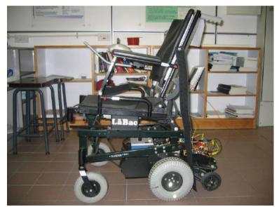
Fig. 9. Prototype of Electric-Powered Wheelchair
