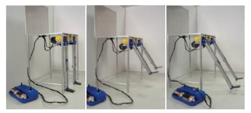
Fig. 23. Motorized foot rest at Fig. 24. Motorized foot rest Fig. 25. Motorized foot rest stationary position after swing angle adjustment after length adjustment
