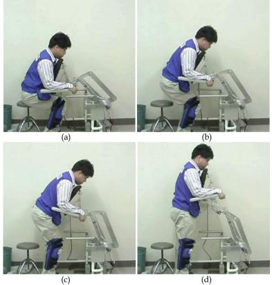
Fig. 15. Standing up motion with our system. (Our proposed scheme) The tester uses wearing equipment for the experience of the elderly (Takeda et al., 2001).
